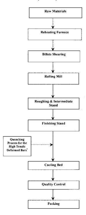
Billets, the raw material required for production of steel bars are procured and tested for quality.
